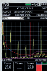
Distance- Amplitude Curves (DAC)
